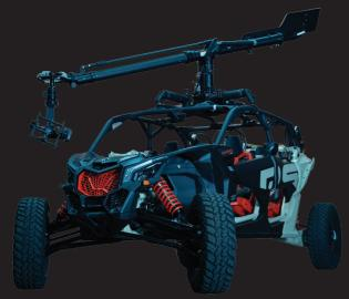
The CLASSIC also has been successfully rigged to an all terrain vehicle like the CANAM Maverick Turbo RR and likewise can be rigged to any off road vehicle for use both moving or static shots with a suitable gimbal (Ronin 2/Movi XL/Movi Carbon).
