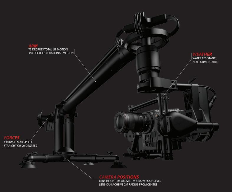
The Motocrane Classic was the first car crane using universal suction mounts to quickly fit the rig to most vehicle roofs' or even the picture car itself for reverse angle shots.
